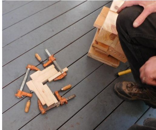
Jig to clamp a 45 corner together. (see page #9)
