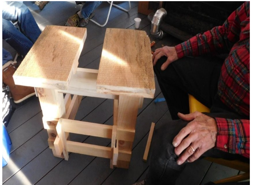
Jig to clamp a 45 corner together. (see page #9)
