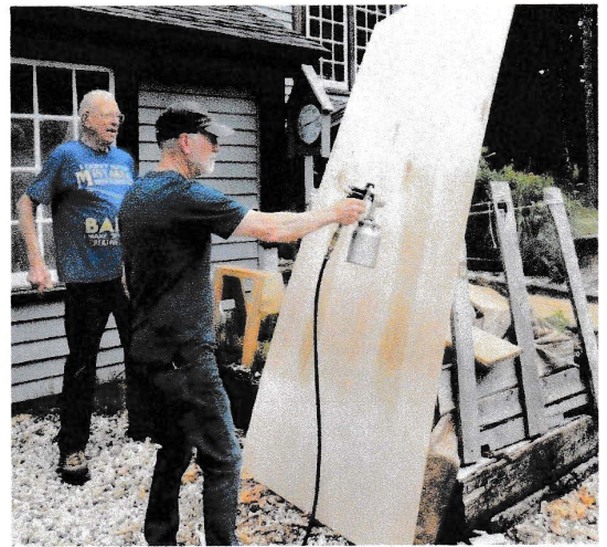
The fearless 4 prepared to do spray finishing. Joe Elichaa, Bob Kearney, Barbara White, Steve Smith. Below: 1st practice spraying water on plywood to obtain wide coverage and even material flow. The skill to spray evenly is arm & hand position, distance from work surface, and travel speed across work
