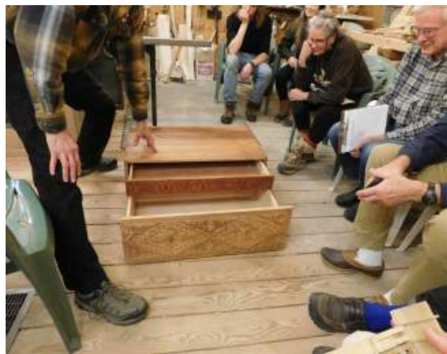
Above: Toolbox base. A drawer within a drawer. This is designed to be a stackable unit.
