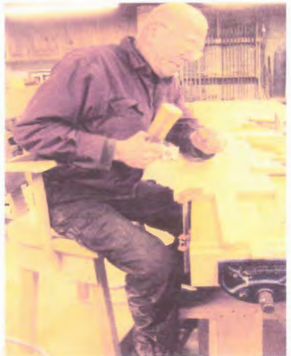
Left: The box shown will be placed beneath a tool chest for additional storage. The large drawer front being carved will fill the opening. The smaller drawer shown fits within the box & behind the large drawer front. When opened, access is gained to the small drawer.
